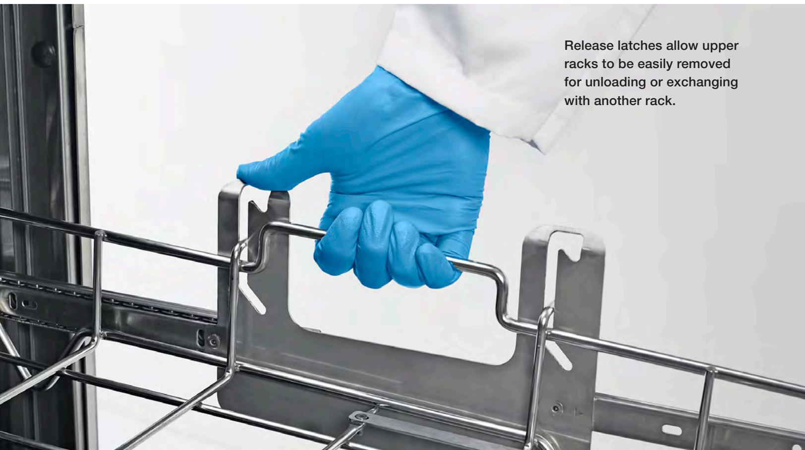
Release latches allow upper racks to be easily removed for unloading or exchanging with another rack.
