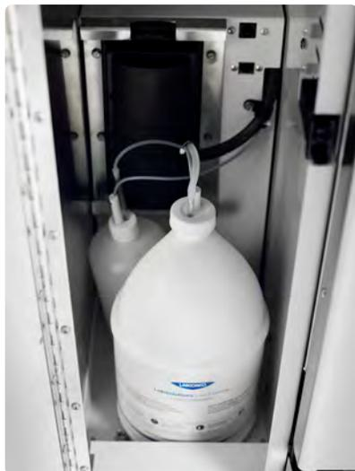
The side compartment of the Reliance 100XLS houses a 99.97% efficient HEPA filter, automatic liquid detergent and rinse aid dispensers.
